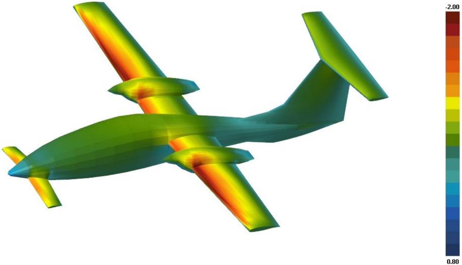
Pressure distribution, angle of attack  $\alpha = 7.5^\circ$
