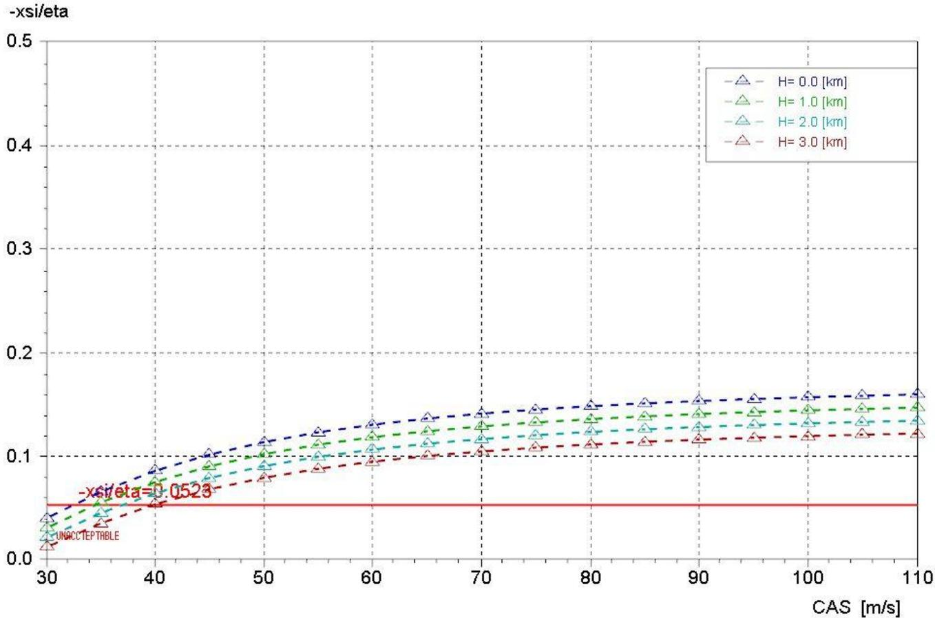
Dutch roll characteristics versus calibrated airspeed (CS-23.181 criterion)
