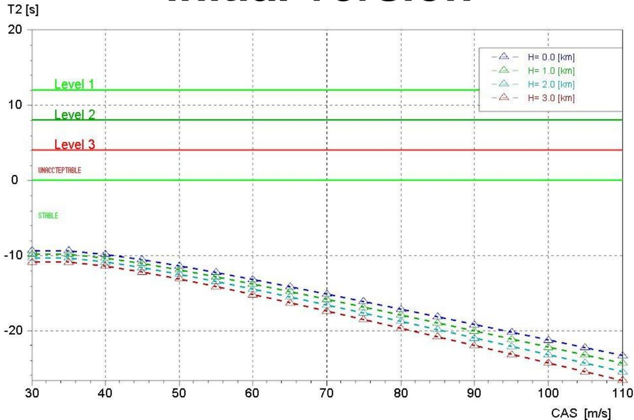
Second essential lateral mode of motion is spiral mode. This mode is stable in whole airspeed range – figure above (MIL-F-8785C criteria).
