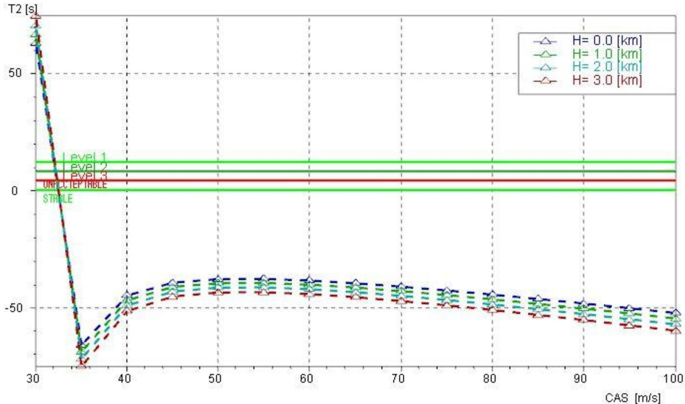
Time to double for spiral mode against background of MIL F-8785C for clean configuration, front CG position criteria
