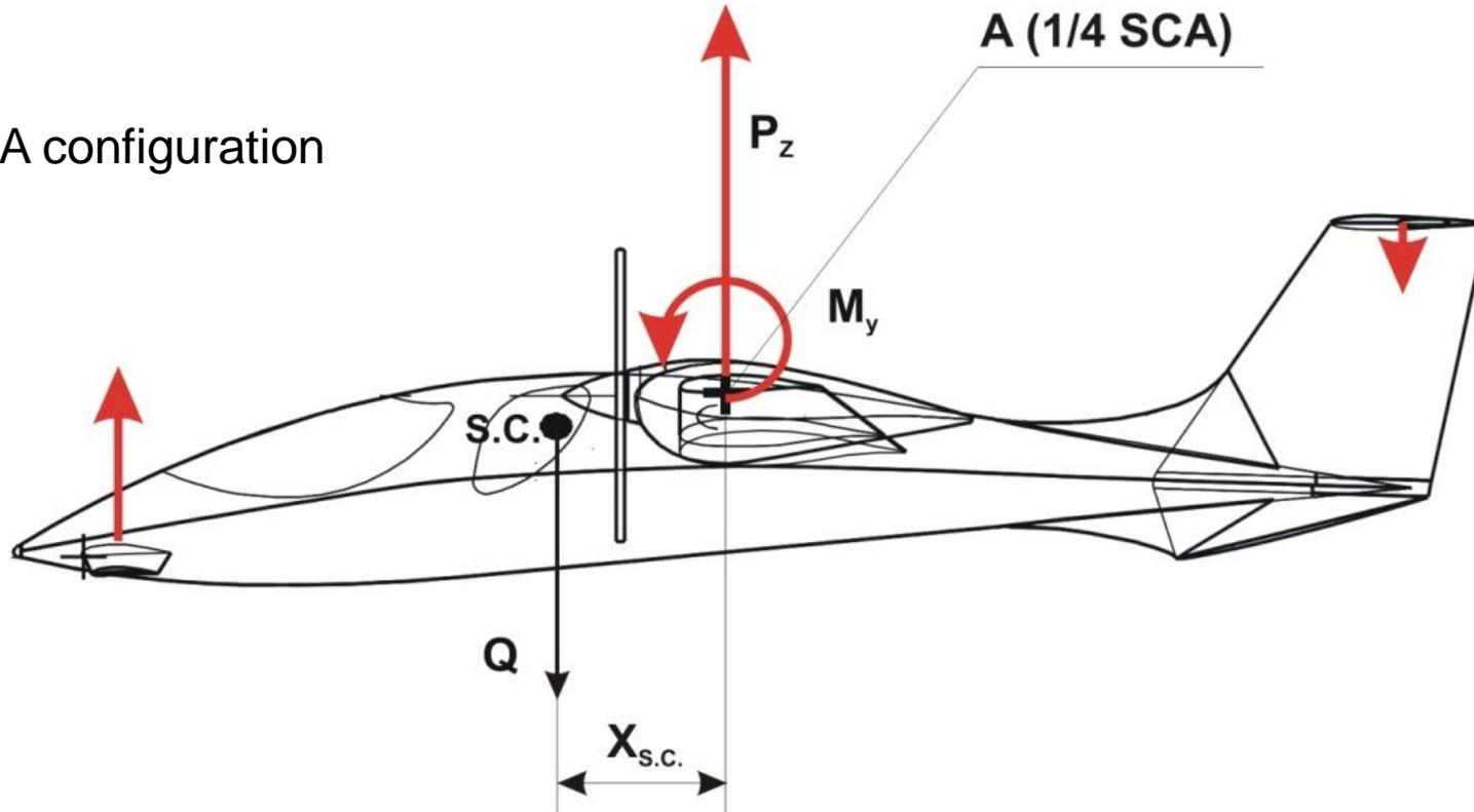
Additional 3<sup>rd</sup> surface decreases negative lift on the horizontal tail and improves the lift balance and classical horizontal tail satisfies longitudinal stability
