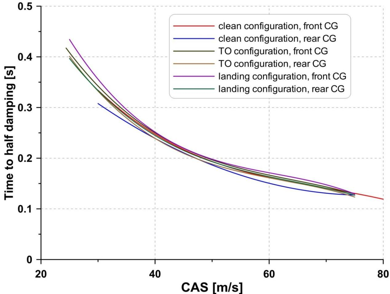
Short Period oscillation - time to half damping versus calibrated airspeed
