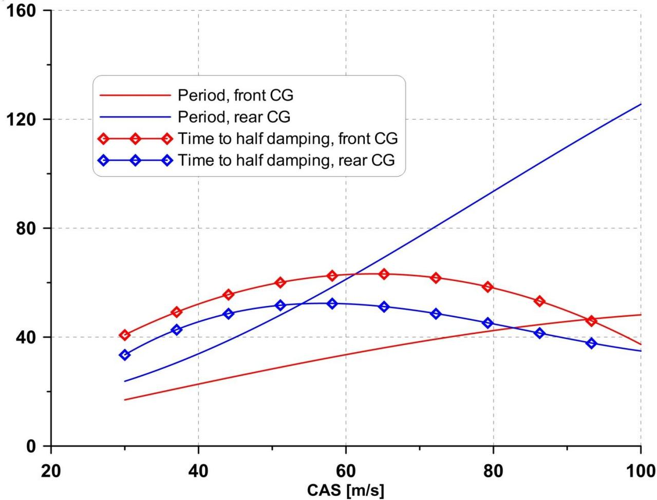
Phugoid - period and time to half damping versus calibrated airspeed
