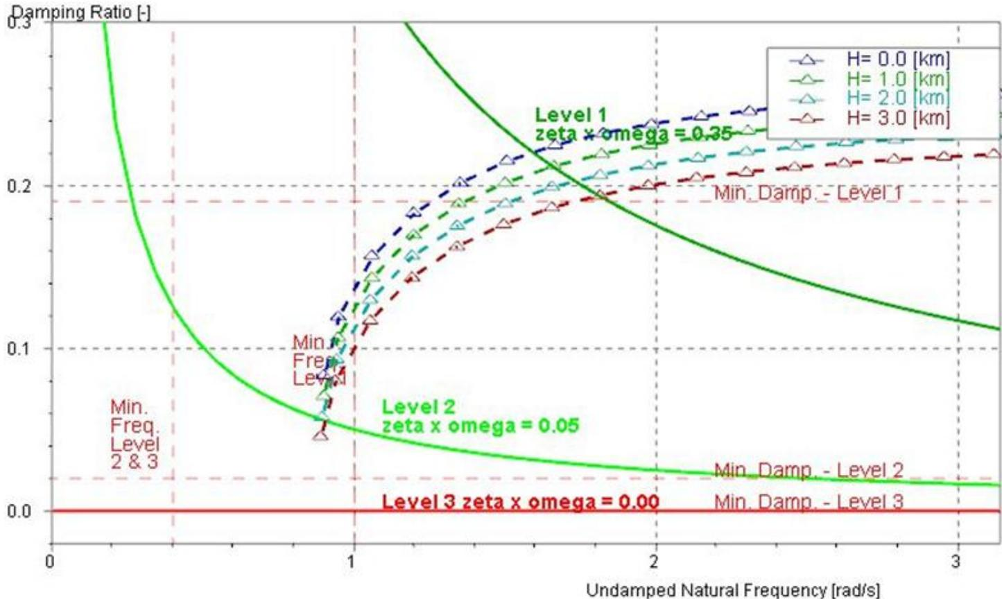
Dutch roll characteristics against background of MIL-F-8785C for landing configuration and rear CG position criteria. It also shows good Dutch roll characteristics, which are in Level 1 & 2 for whole flight envelope.
