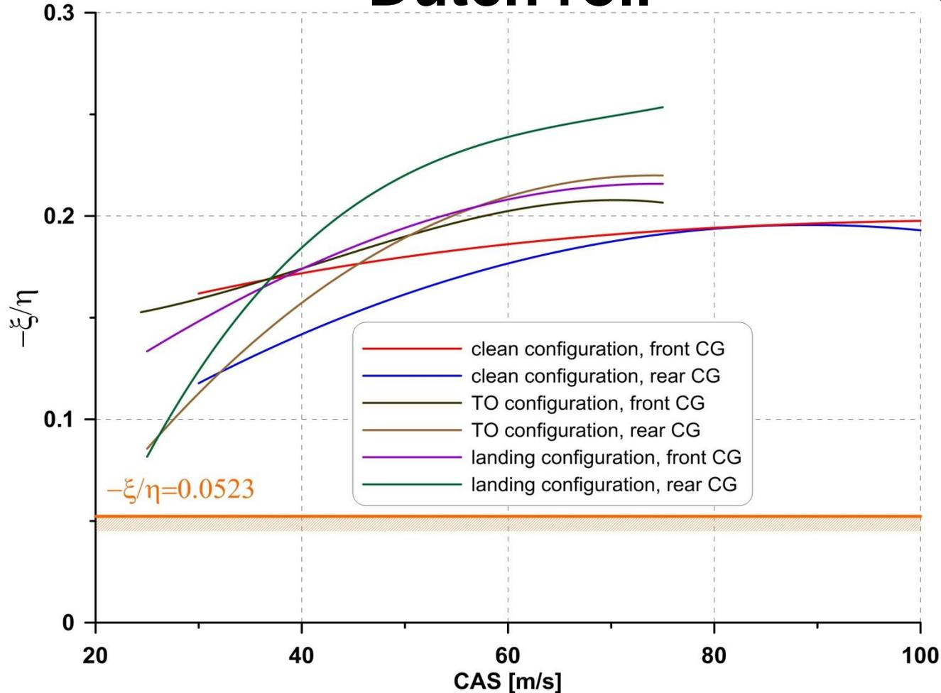
Dutch roll characteristics versus calibrated airspeed (CS-23.181 criterion)
