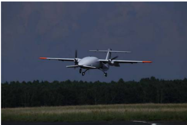
Figure 15 Test flight of 40 per cent scaled model
